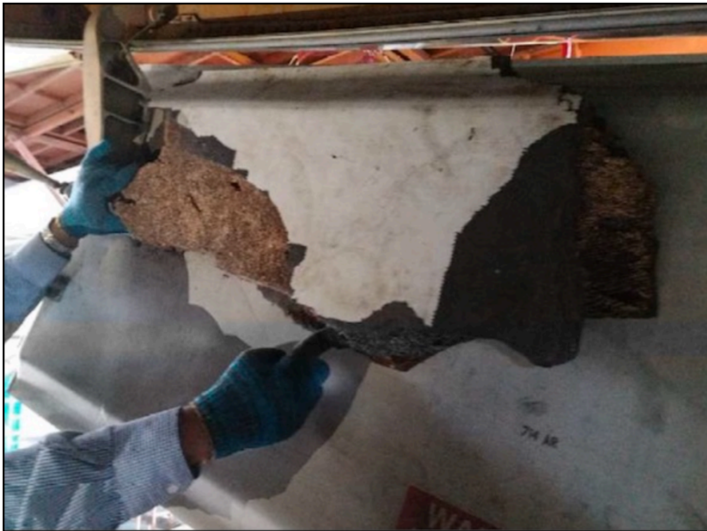
Figure 35: Nose Wheel Door Debris found 12 th June 2016 in Antsiraka Beach, Madagascar.
