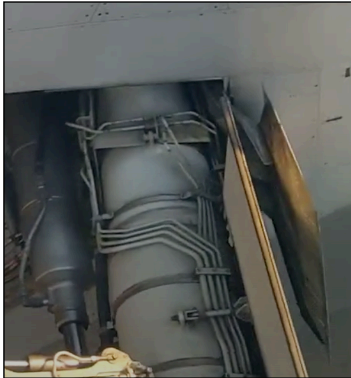
Figure 50: Close Up Main Landing Gear Trunnion Door Right Wing.
