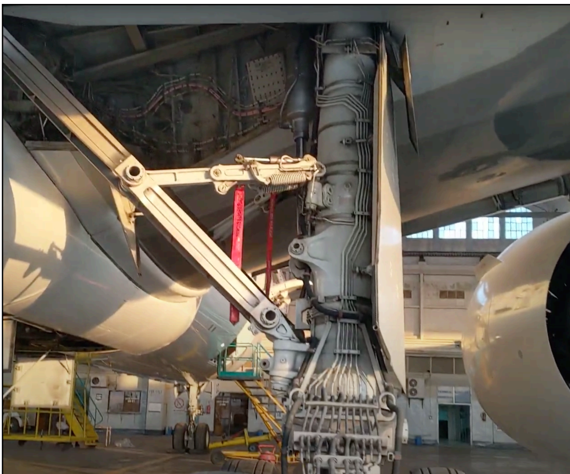
Figure 44: Boeing 777-200 Main Landing Gear Doors.
