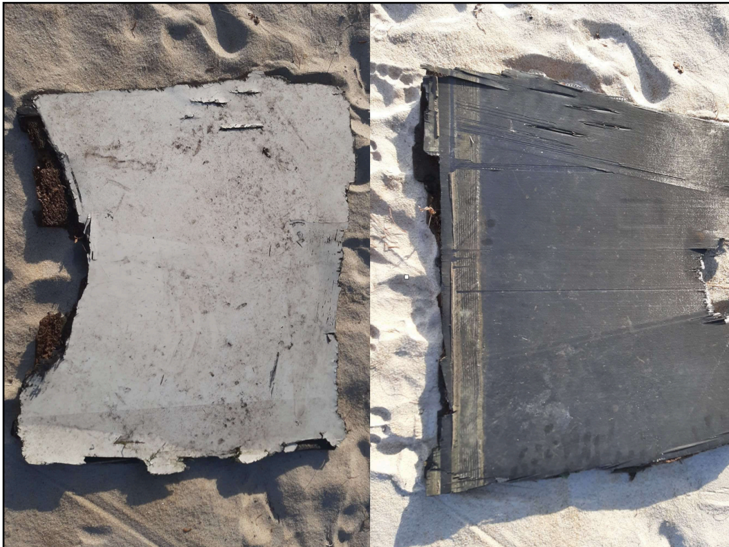
Figure 25: Debris Item with puncture damage both sides.
