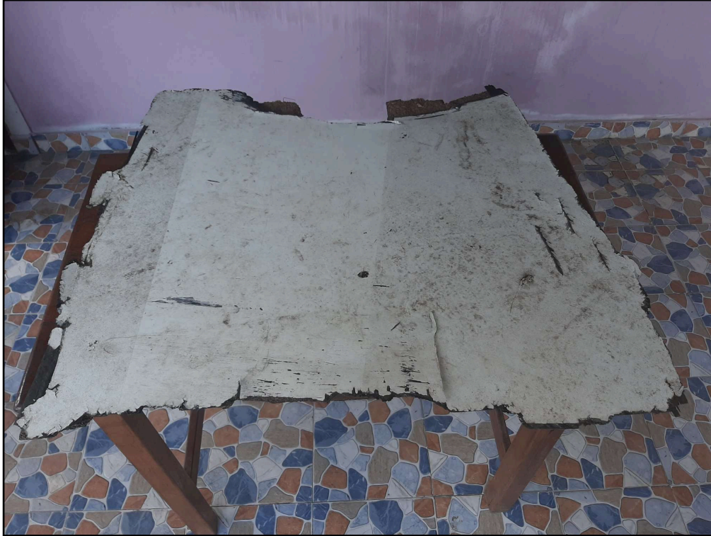
Figure 23: Debris Item White Side with tears and circular marking.
