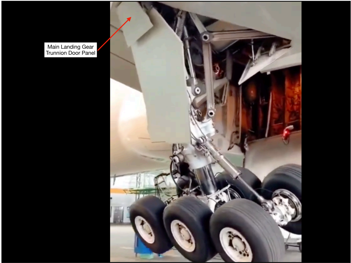
Figure 56: Boeing 777-200ER Left Wing Main Landing Gear Trunnion Door Panel.
