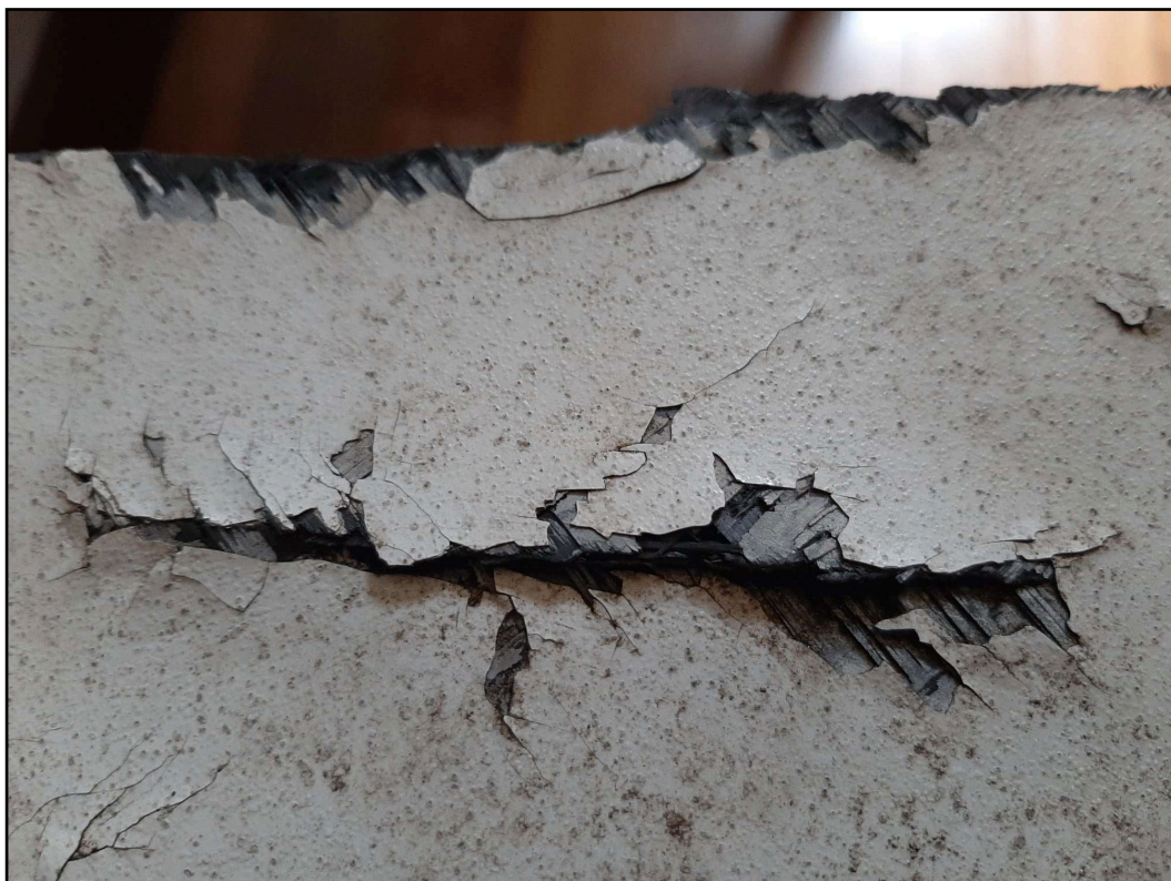
Figure 30: Close up of the lifting of the surface of the white side with shadows.
