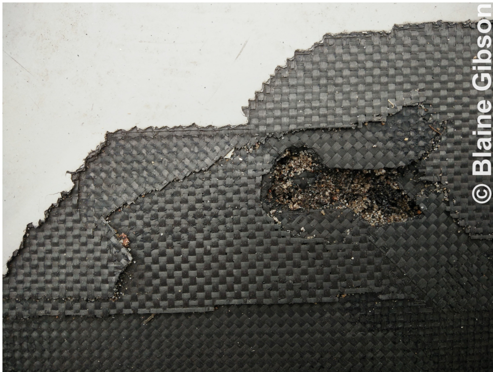
Figure 38: Nose Wheel Door Debris showing puncture damage.
