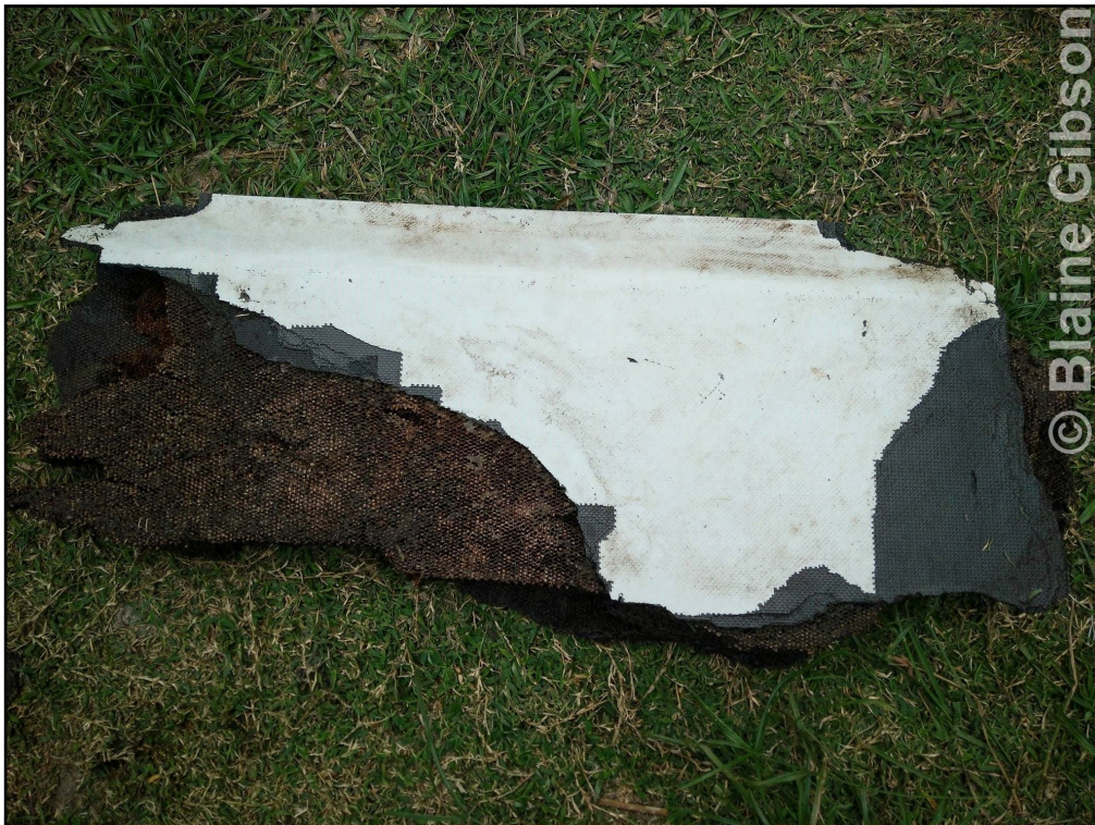
Figure 36: Nose Wheel Door Debris showing tension damage and partial delamination.
