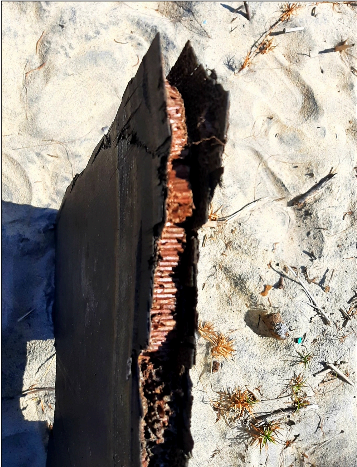
Figure 10: Debris Item Honeycomb Sandwich.
