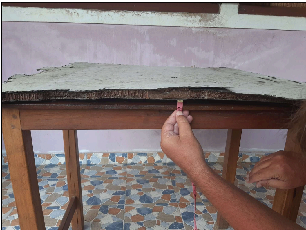
Figure 12: Debris Item Side View with maximum 3/4" curvature.
