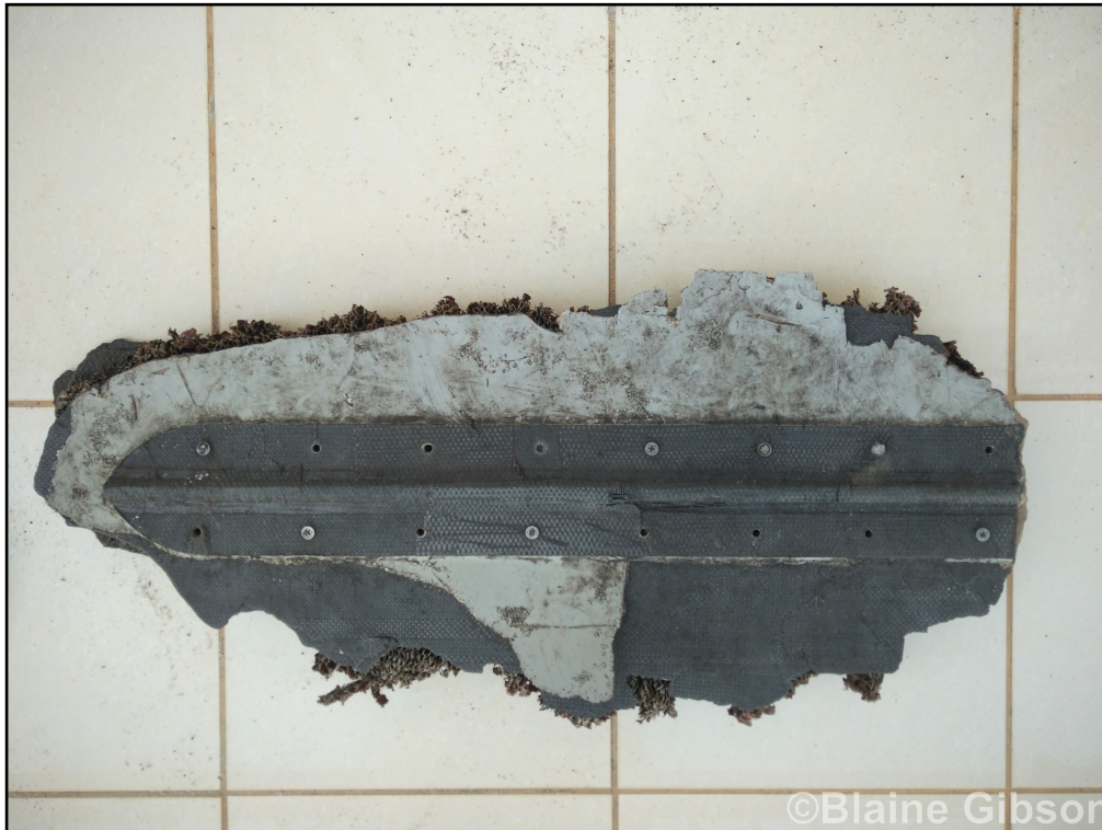
Figure 41: Vortex Generator showing partial delamination.
