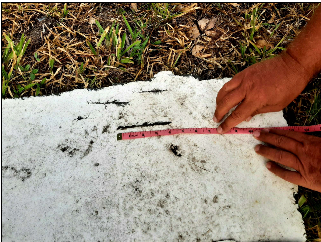
Figure 26: Puncture damage position 13" from the edge.
