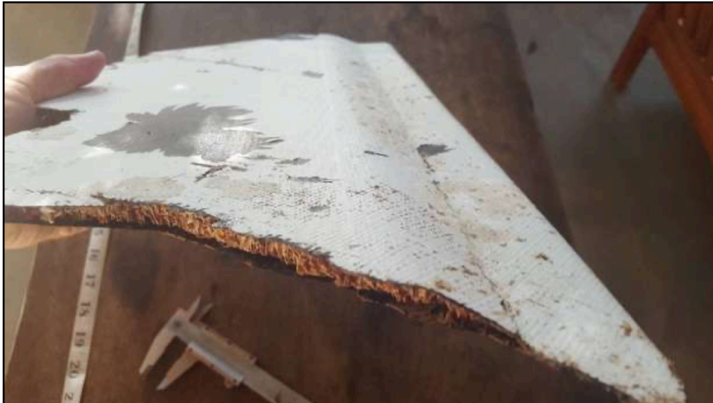
Figure 33: Wing to Body Fairing found 30 th April 2016 in Chemucane, Mozambique.
