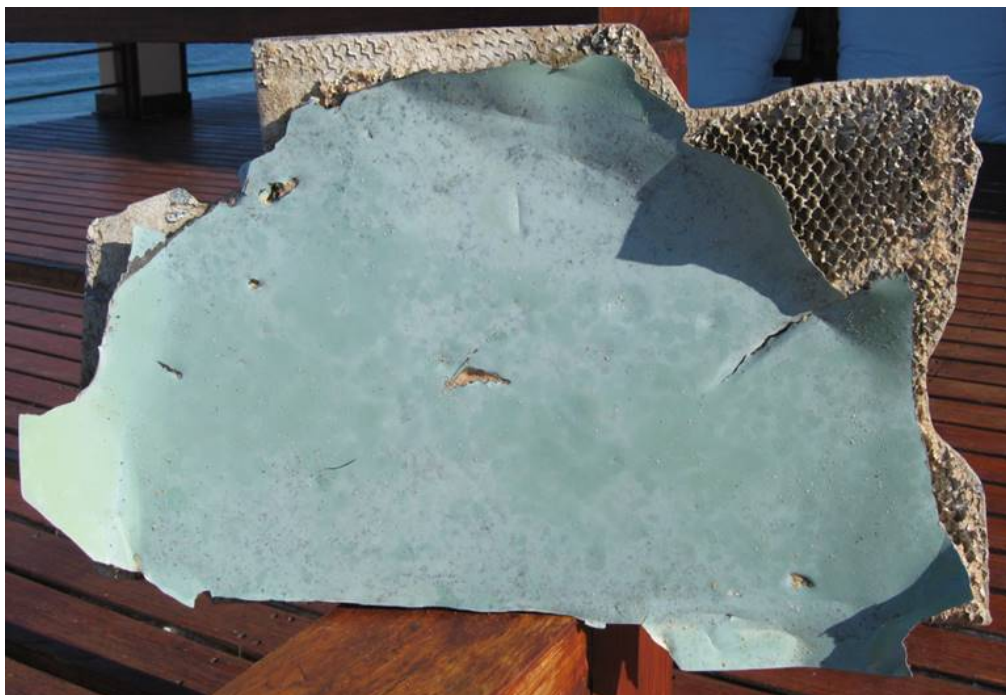
Figure 40: Panel Debris showing partial delamination.
