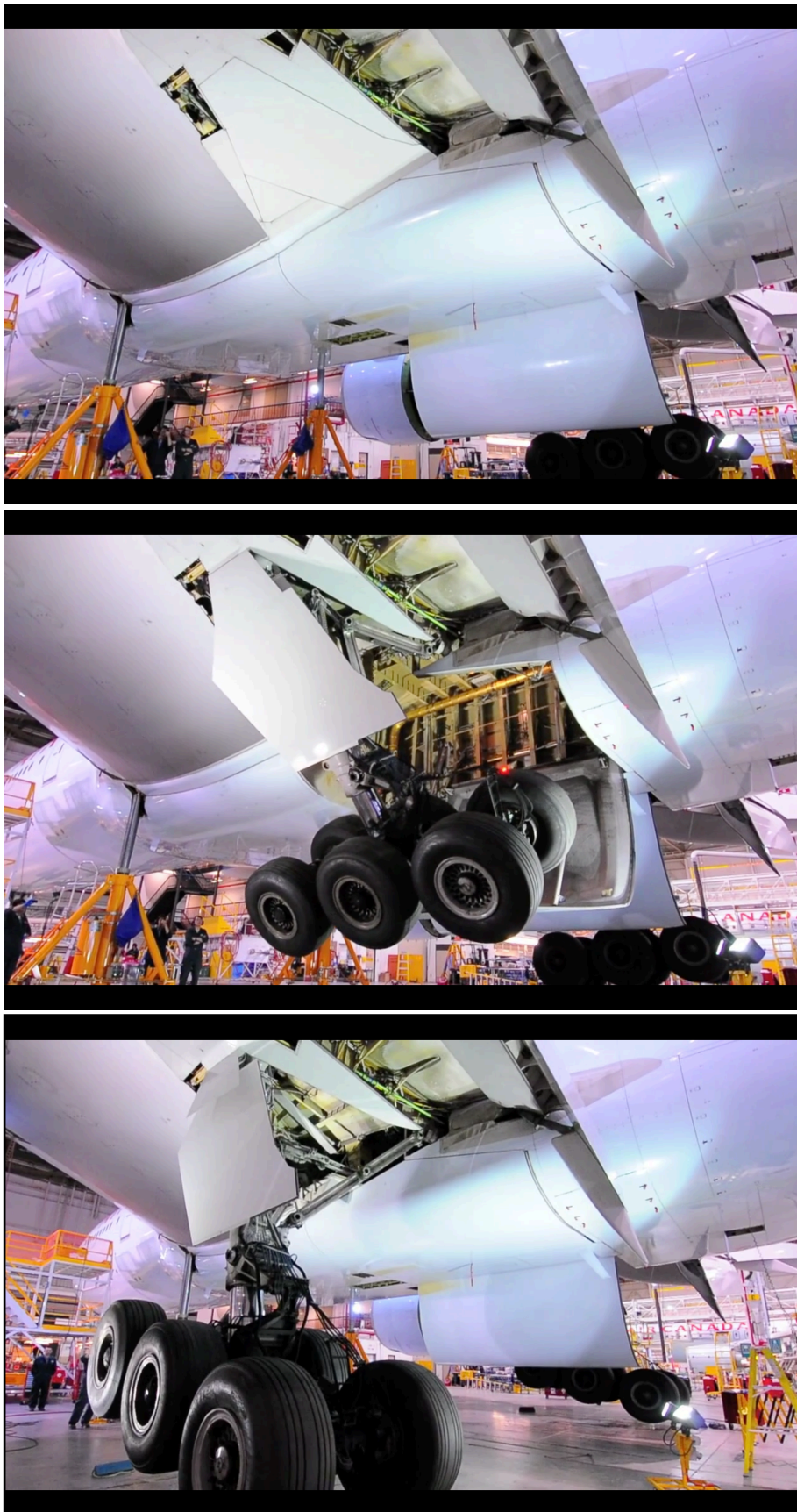
Figure 47: Main Landing Gear Doors Opening Sequence.
