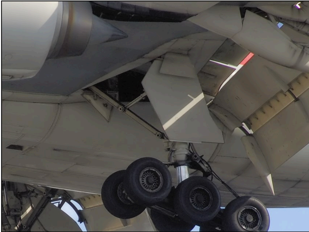
Figure 45: Main Landing Gear Doors with Under Carriage Extended Left Wing.
