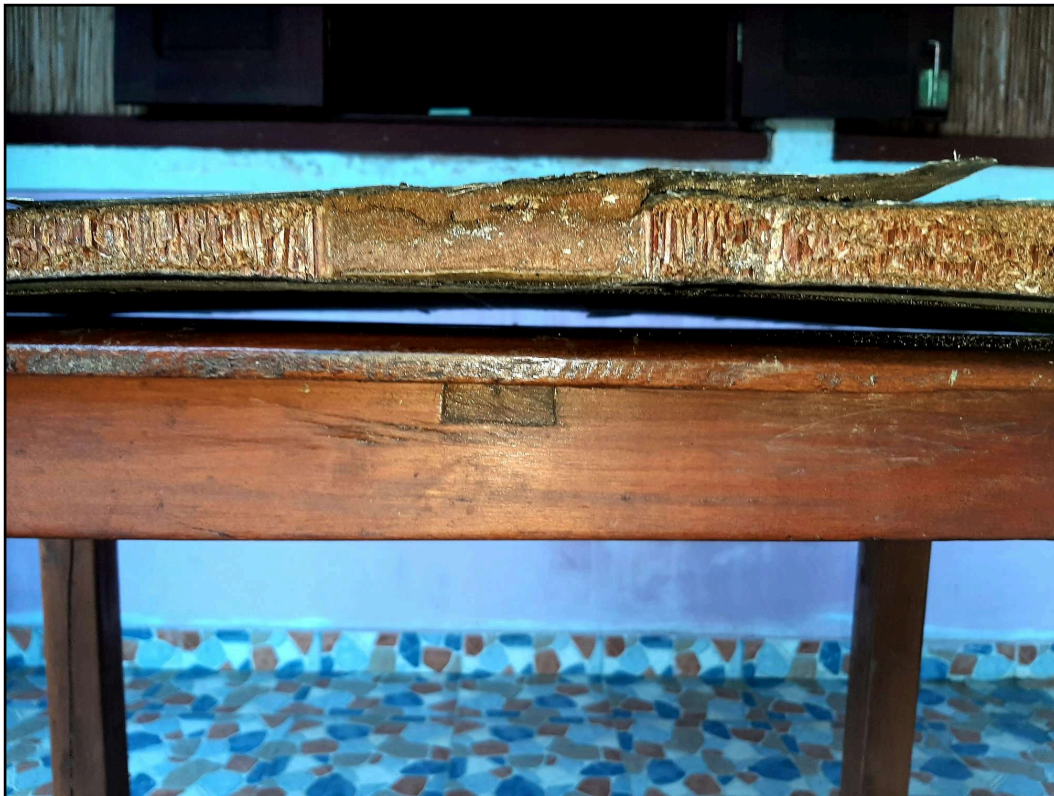
Figure 13: Debris Item Side View with honeycomb and a more solid fill.
