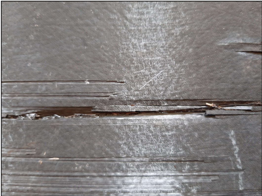
Figure 32: Close up of the largest indentation of the surface of the black side.
