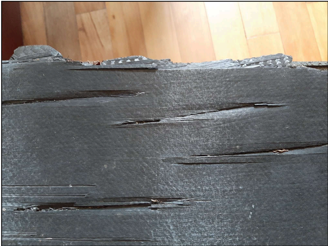
Figure 31: Close up of the indentation of the surface of the black side.
