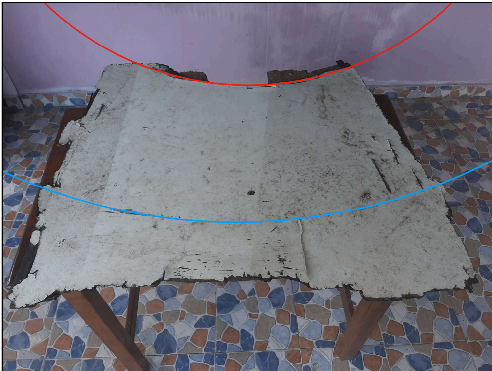
Figure 24: Debris Item White Side with tears and circular marking (photo enhanced).
