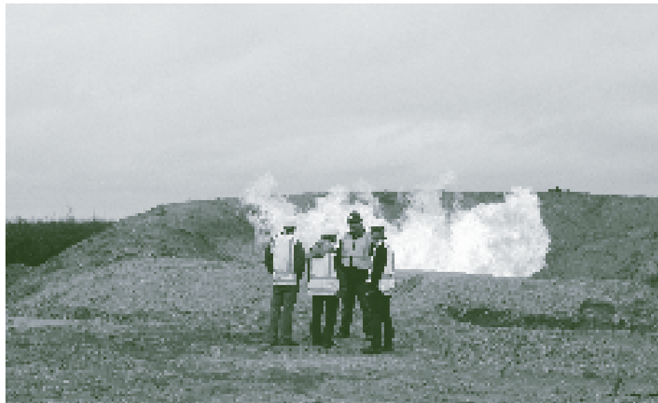
Figure 5.3 Pre-production gas is flared in a pit at TAG Oil's Cheal-C well site. Flare pits often capture wastewater as gas is burned off.
