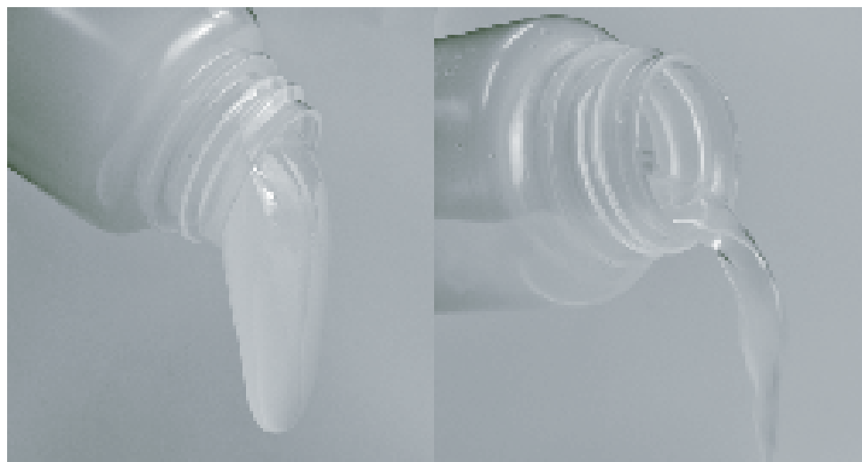
Figure 4.6 The fracking fluid is pumped into the well in a jelly like state (on the left). Once underground the temperature triggers the gel to break down into a liquid (on the right) to make it easier to return to the surface.
