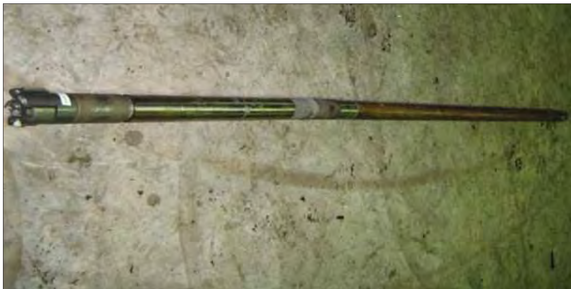
Figure 9.2: Bit, down-hole motor and assembly 33
