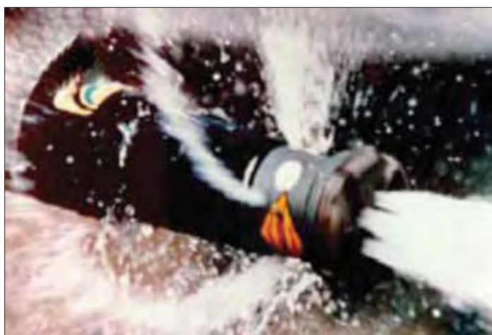
Figure 9.3: Rotating drill bit with high-pressure water 34
