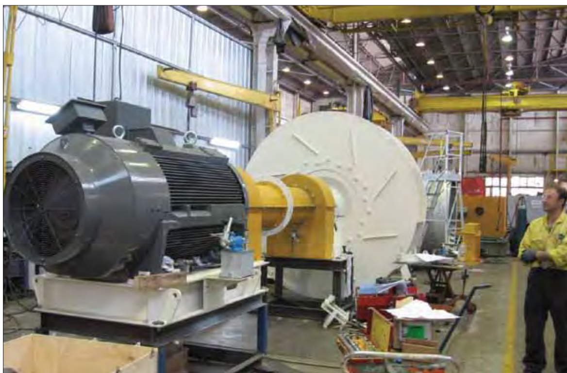
Figure 8.8: Underground fan being assembled in factory
