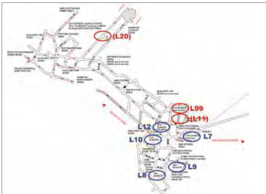
Figure 10.1: Location of fixed methane sensors 22
