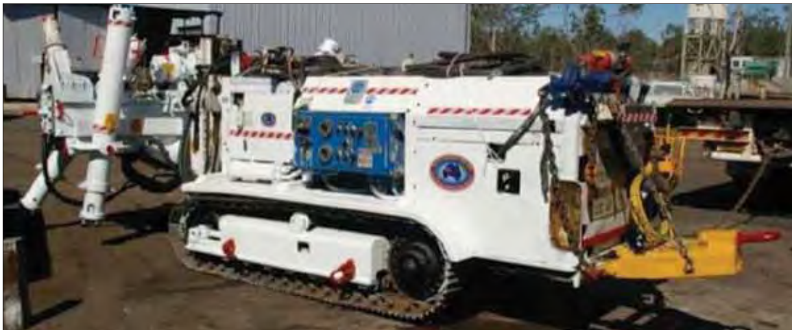
Figure 9.1: Track-mounted Boart Longyear LMC75 drill rig 31
