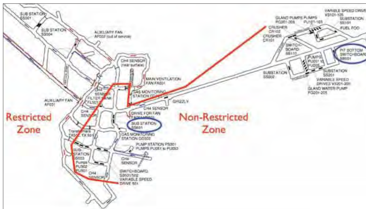
Figure 11.1: Main electrical area and zones underground 2
