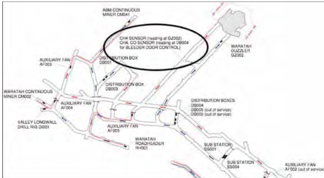
Figure 10.3: Location of hydro-panel sensors 29
