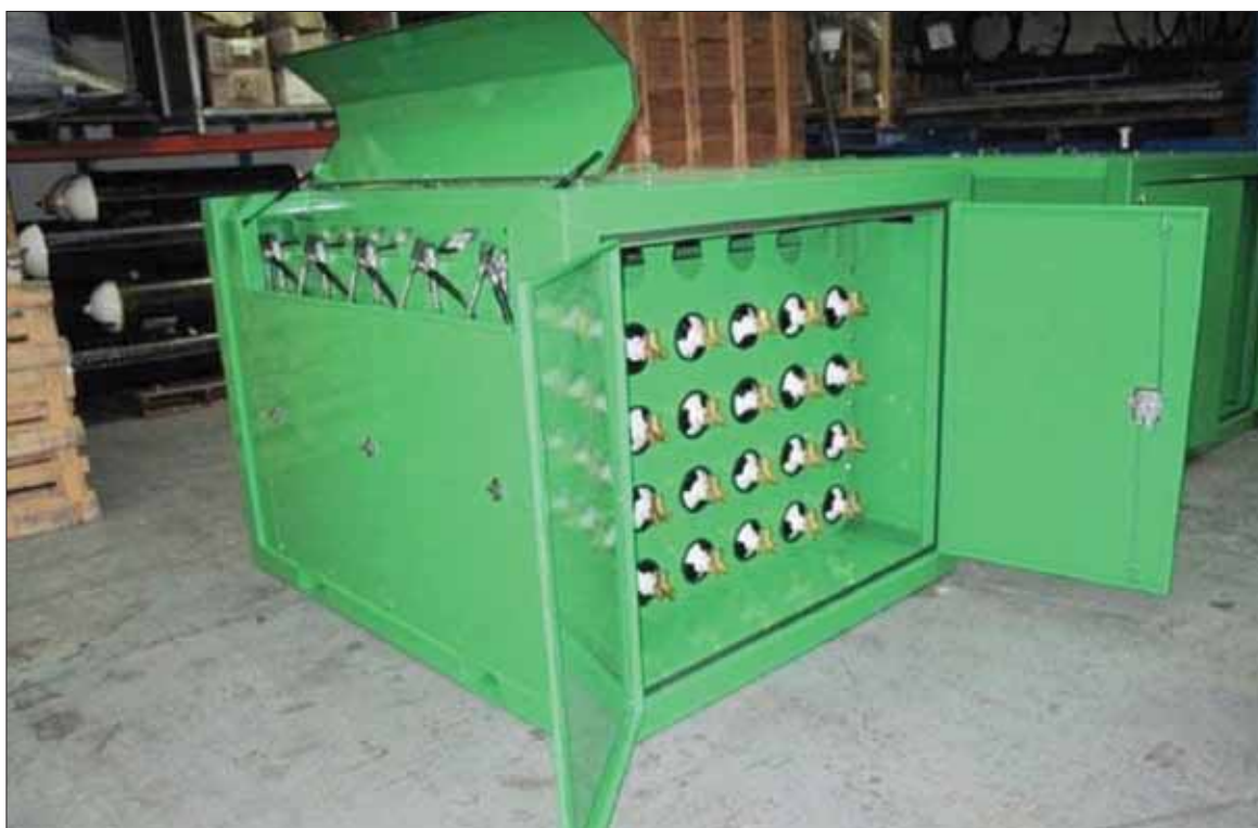
Figure 33.3: Recharge station for compressed air breathing apparatus
